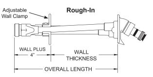
Overall Length = Wall Thickness + Inlet Close Coupled Overall Length = 5"
